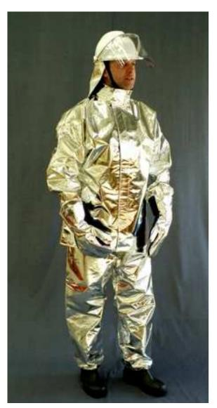
The Flameguard Mk 3 suit is a two-piece garment constructed in aluminised fire resistant modacrylic cotton to EN11612. The jacket has a stand-up collar, elasticated cuffs, and is closed by 50 mm wide touch and close fastening to the front and collar. The trousers have 25 mm webbing braces with plastic adjusters to fit a wide range of wearers. The lower leg is elasticated.
