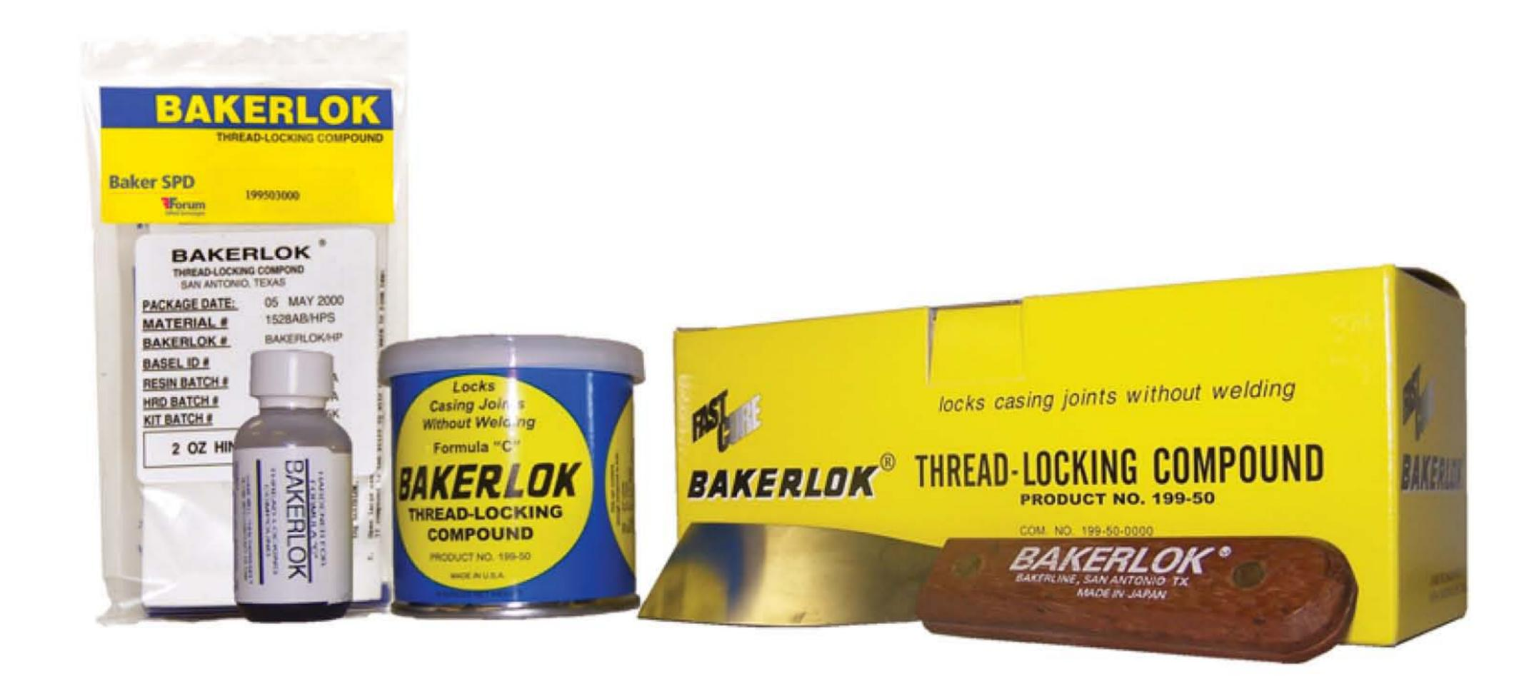
Fast Cure Bakerlok® Thread-Locking Compound replaces welding for casing joints on the bottom lengths to prevent unscrewing while drilling out cement. Welding of shoes, couplings, and collars to casing often weakens the casing and should be avoided wherever possible.
