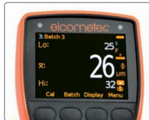
Scan Mode* stores the average, highest and lowest readings over a test area
